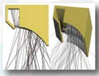
Light distribution by CAE simulation 照射平面光分佈模擬圖
