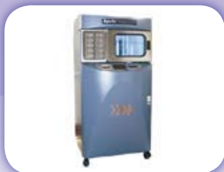
Apollo2 - Xenon Arc Light and Weather Fastness Tester 氙氣弧光燈日晒及氣候牢度試驗機
