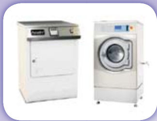
Wascator and Accurdry2 歐標縮水率試驗機及乾衣機
