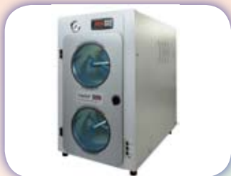
Impulse2 - Random Tumble Pilling Tester 亂翻式起毛及起球測試儀
