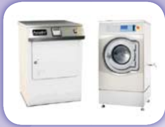
Wascator and Accurdy2 歐標縮水率試驗機及乾衣機
