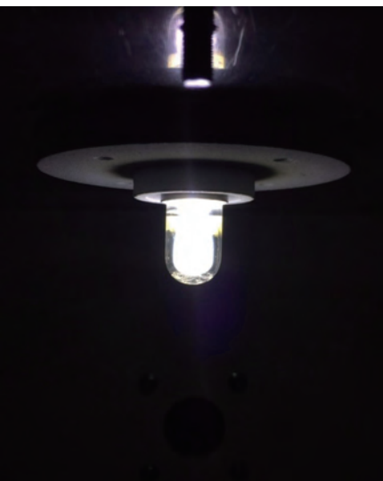
等離子燈內的等離子體電弧 Plasma arc inside the Plasma Light
