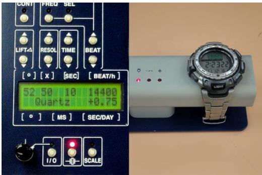
Figure 2-5. Calibration of Watch Testers
