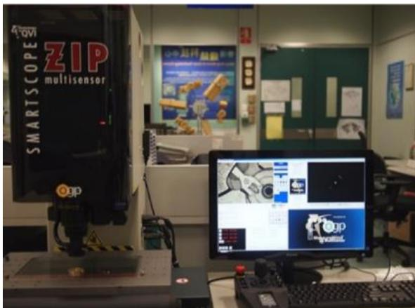
Figure 2-6. Movement component measurement equipment
