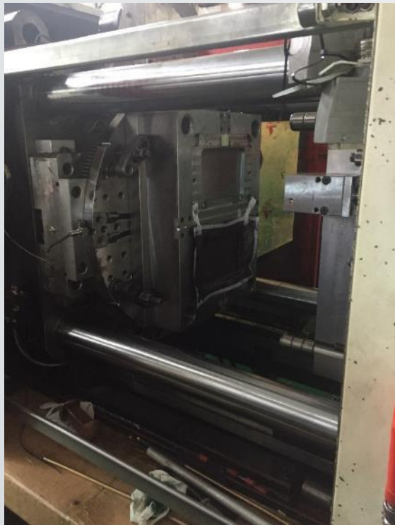
1: Placing of carbon fibre fabric for RTM 2: Mould close for RTM of epoxy resin
