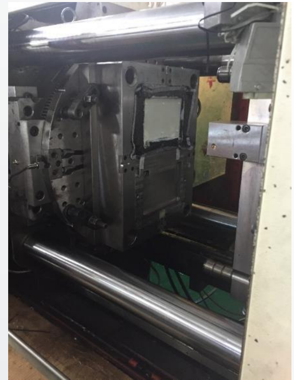
3: Injection moulding of thermoplastic parts onto Epoxy-Carbon fibre composite part
