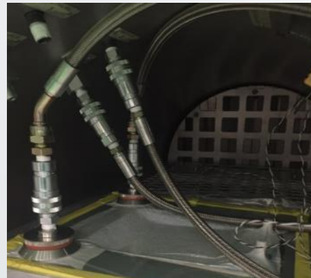
Vacuum applies and curing under pressure and elevated temp
