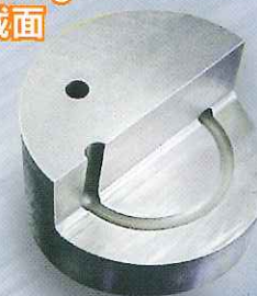
Sectioned Tooling Surface After Diffusion Bonding 焊接後的截面
