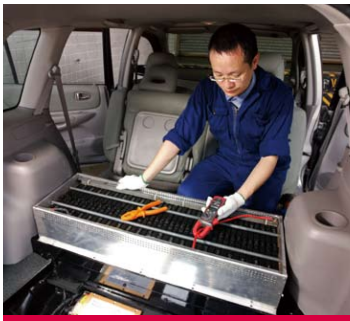
Mr Desmond Liu, Consultant, Environmental Management Division, HKPC, installs a battery on a hybrid electric vehicle jointly developed by HKPC and its industry partners to improve fuel efficiency and reduce emissions.
