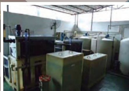
在線回收系統大幅減少蝕刻液耗用及廢液處理費用。 In-line recovery system helps PCB manufacturer reduce consumption of fresh etchant and disposal costs.
