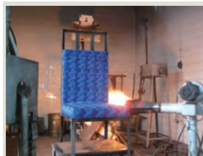
座椅原型進行易燃性測試。 The aircraft seat prototype was undergoing a flammability test.
