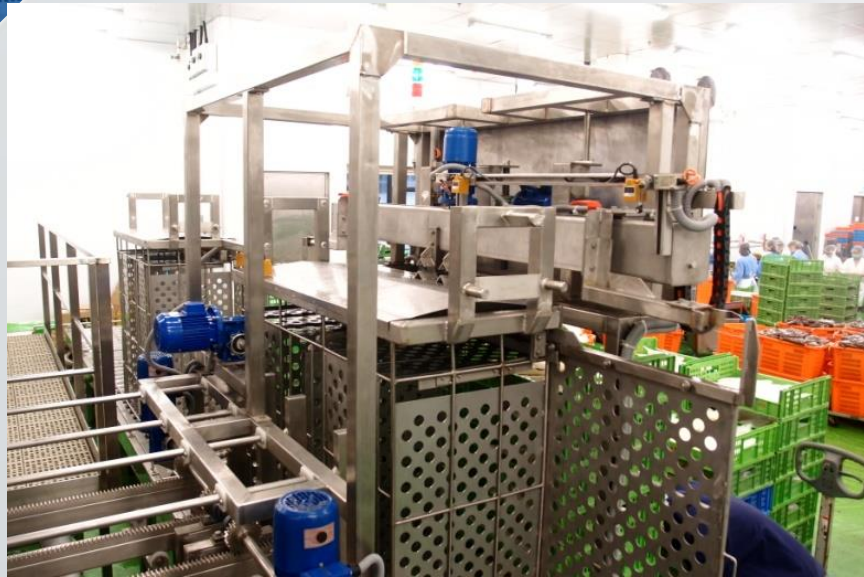
Automatic door opening and output system
