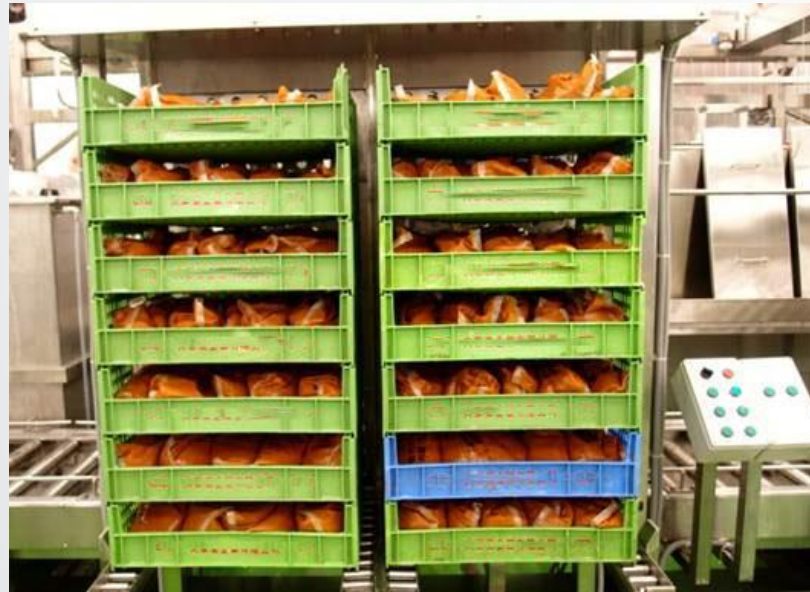
Each submerging basket holds 7x2 trays
