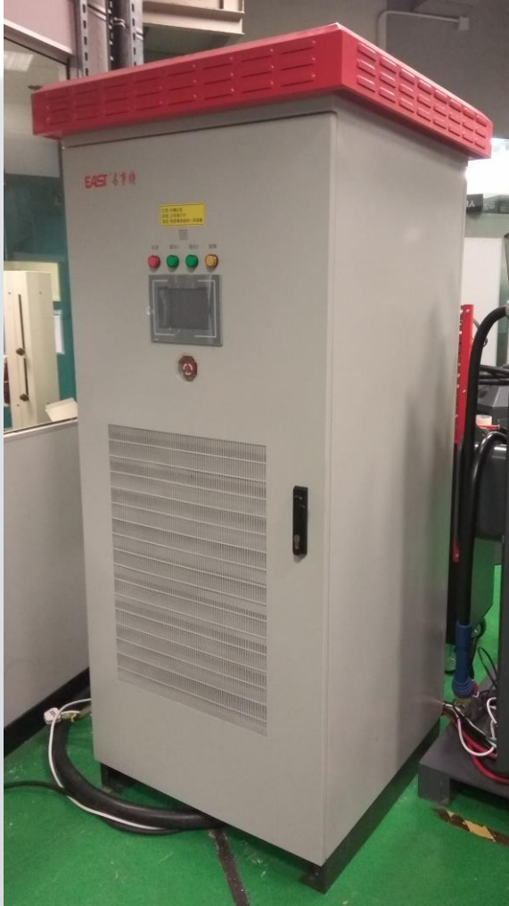
Main Power Converter Dimension: 100 x 80 x 180cm
