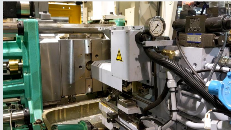
Step 3 – injection of metal layer
