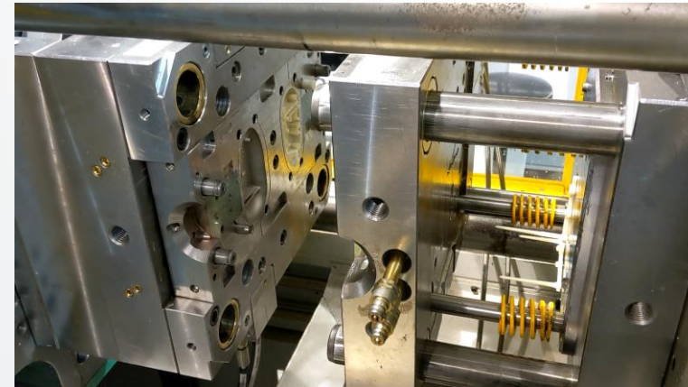
Step 2 – transfer of plastic preform
