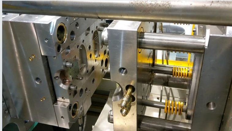
Step 1 – injection of plastic preform in cavity 1
