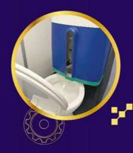
IoT- enabled Smart Toilet Bowl Cleaning System for Public Toilets (Co-developed with EMSD) 智能洗手間清潔機械人 (與機電工程署合作攜手研發項目)
