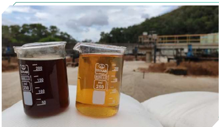
比較已採用(左)和未採用(右)嶄新化學處理方法的堆填區垃圾滲濾液顏色 Comparison of the colour of landfill leachate with (left) and without (right) the Novel Chemical Treatment Process
