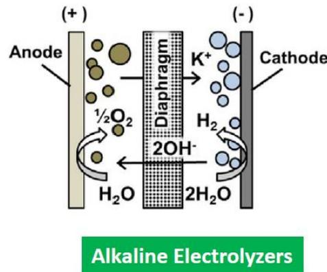
**Figure 5** Cross-sectional view of alkaline electrolyzers
