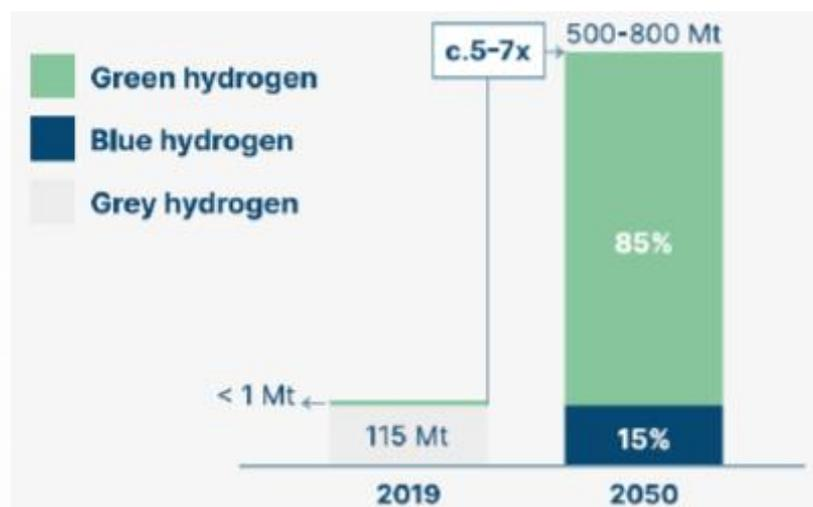
**Figure 2** Multiple-fold increase in clean hydrogen production by 2050. Source: ETC (2021) *Making the Hydrogen Economy Possible*.
