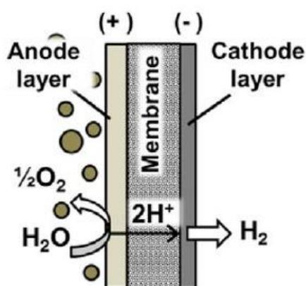
**Figure 6** Cross-sectional view of PEM electrolyser
