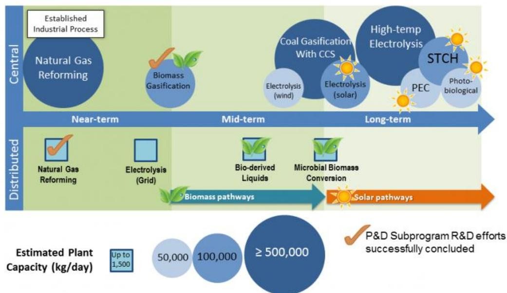
**Figure 7** Near-term, mid-term and long-term technologies for hydrogen production.
